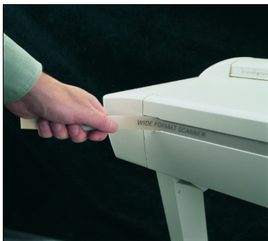
Figure 6-1 Access the DIL-switches
